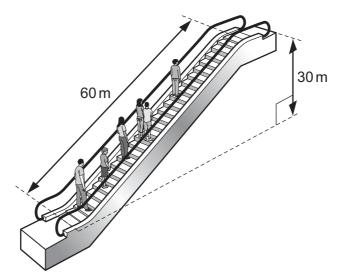
To drive the escalator against the forces of friction when there are no passengers requires a power of 2.0 kW.
