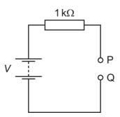
A student attempts to measure the potential difference (p.d.) between points P and Q using two voltmeters, one at a time. The first voltmeter has a resistance of  $1 \text{ k}\Omega$  and the second voltmeter has a resistance of  $1 \text{ M}\Omega$ .
