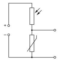
Under which set of conditions will the potential difference across the thermistor have the greatest value?
